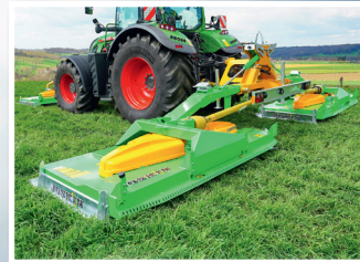
Possibility of adding 2 rear mowers to cover a width of 7.50m
