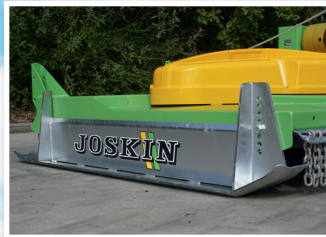
Equipped with 2 XXL skids to ensure a perfect glide of the machine
